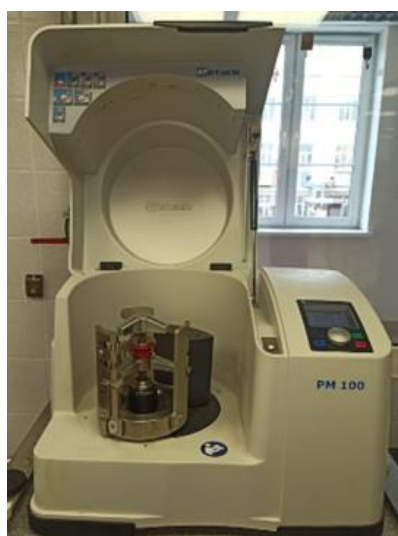
Figure 1. The photo of the ball-mill Retsch PM100 used in this research
