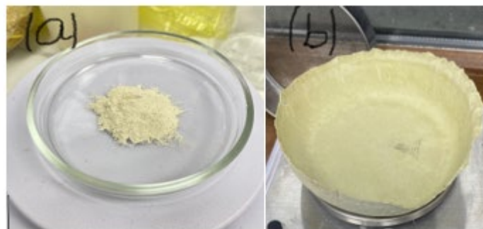
Fig 1. - Material and Final Product: (a) Eggshell Powder; (b) Plate from Lawn Grass without Coating.
