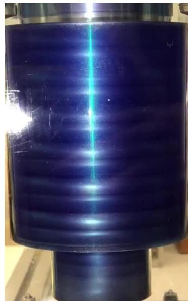
Figure 4. Flow pattern with 393,6 rpm angular velocity
