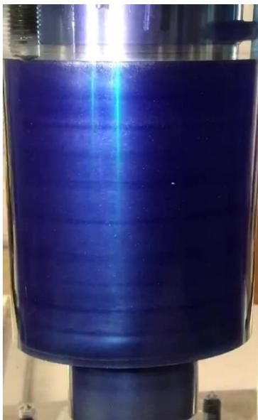
Figure 3. Flow pattern with 184,2 rpm angular velocity
